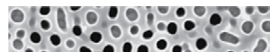
A scanning electron micrograph of Singular ID fingerprint technology. The fingerprint consists of micro- or nanoscale features embedded within a material. Each fingerprint produces its own unique signal and even we are unable to reproduce a fingerprint.
